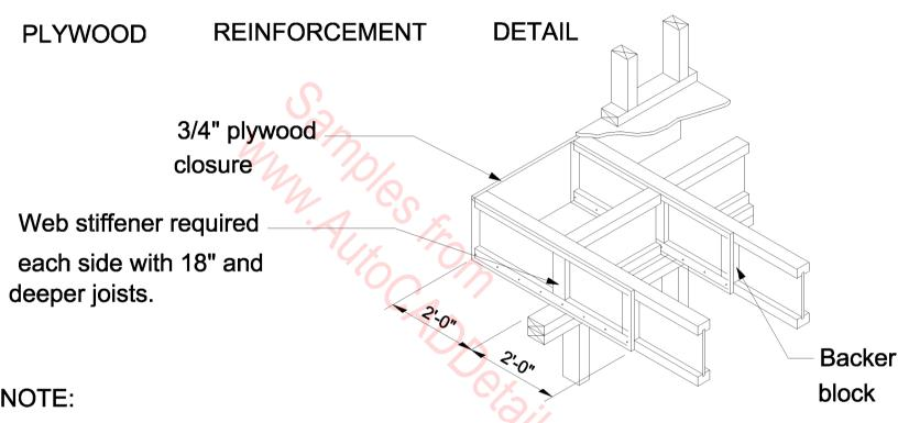
3/4"x48" CDX plywood reinforcement or other 3/4" APA 48/24 rated sheathing must match the full depth of the BCI joist. Nail to the BCI joist with 8d nails at 6" o.c. and nail with 4-8d nails into backer block. When reinforcing both sides, stagger nails to avoid splitting. Install with face grain horizontal.
